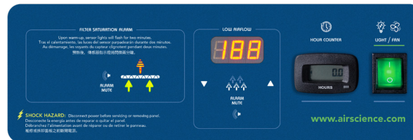
FSA/AutoCAL Control Panel
