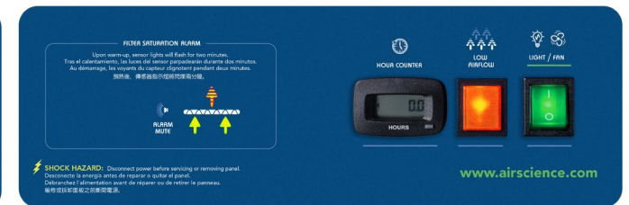
FSA Control Panel (FSA)
