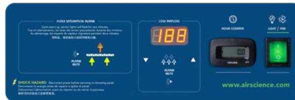
FSA/Autocal Control Panel
